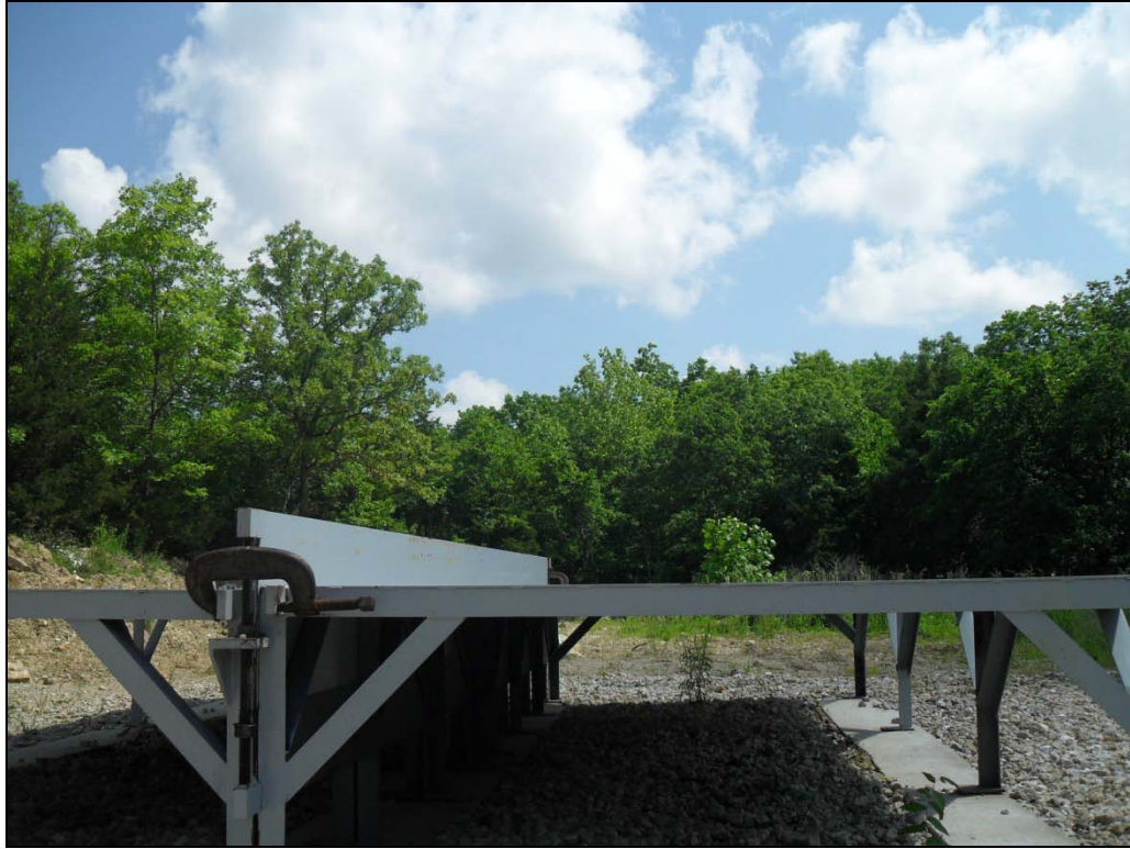
Figure 3.7. Blast table with wall height of 226 mm.
